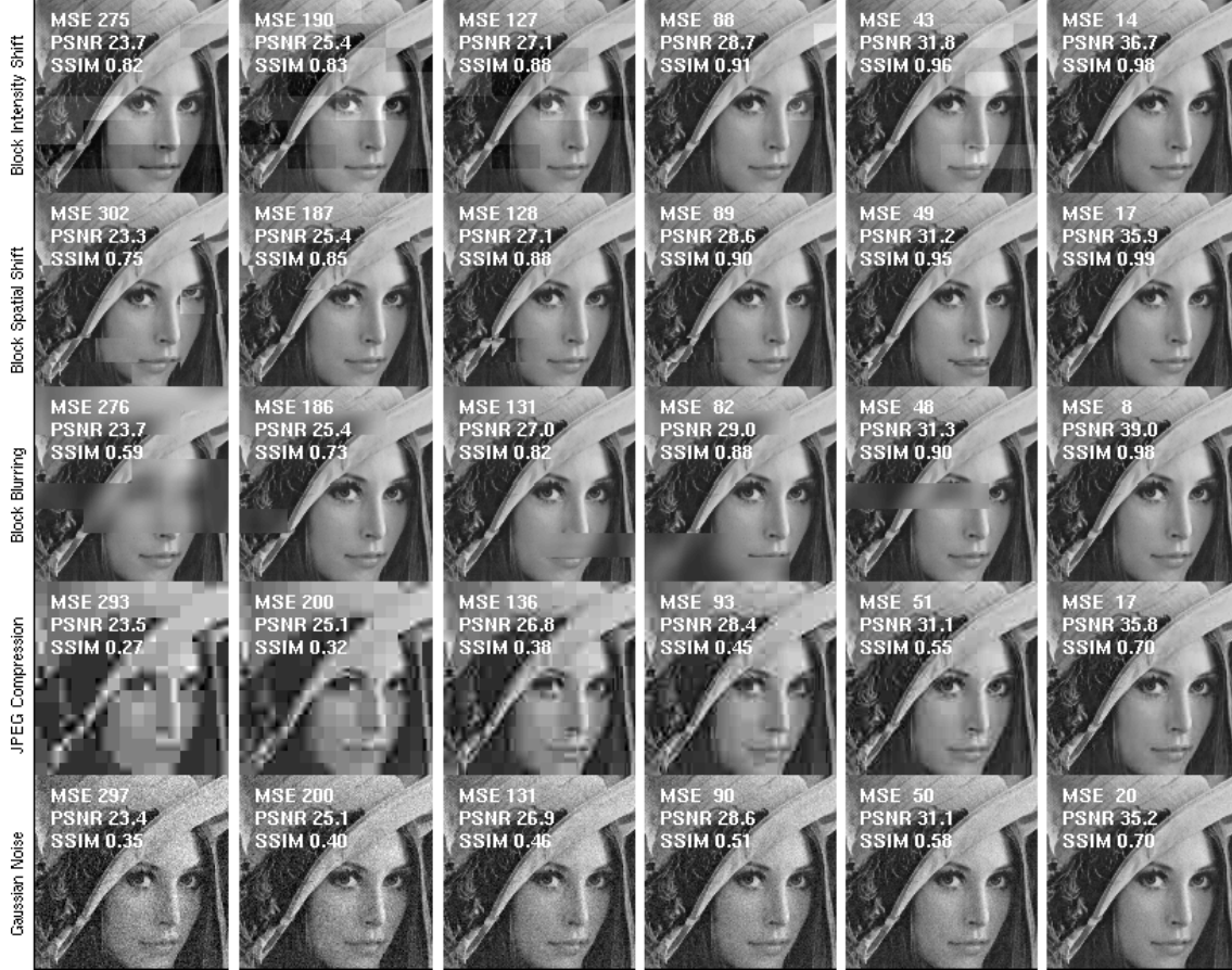
Figure 5. Example realistic distortion images where columns have approximately equal mean-squared error. From bottom to top, the lower two rows are baseline images with distortions created by (1) adding white noise and (2) JPEG compression, while the upper three rows result from application of our probabilistic model with (3) block blur, (4) block spatial shift, and (5) block intensity shift distortions. The cropped central 128x128 region of the images is shown, labeled with MSE, PSNR, and CWSSIM results.
