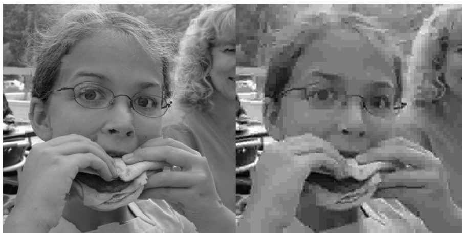
Figure 7. Spatial shift image (left) versus DCT quantization image (right) with equal MSE=100 and CWSSIM of 0.78 and 0.30, respectively. CWSSIM agrees with the subjective observation that the left image has much higher perceptual quality than the right image.
