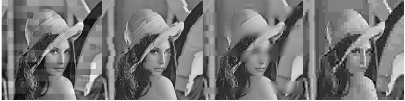
Figure 6. Four degraded images with approximately equal MSE. From left to right, the distortions are: block intensity shifts, block spatial shifts, block blur, and DCT coefficient quantization. These images correspond to the left column of Figure 5.
