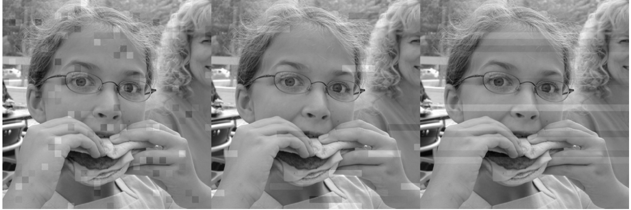
Figure 8. Effect of MB grouping parameter— M blocks per packet—for equal MSE=50 . From left to right, M = 1, 5, and 32 (entire row) while CWSSIM=0.91, 0.96, and 0.94, respectively. CWSSIM agrees with the subjective observation that the center image has higher perceptual quality than the others.
