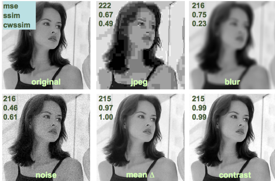
Figure 1. The effect of suprathreshold distortions on MSE, SSIM, and CWSSIM metrics. SSIM and CWSSIM correspond well with the intuitive idea that changes in lighting (mean and contrast) have very little effect on image quality.
