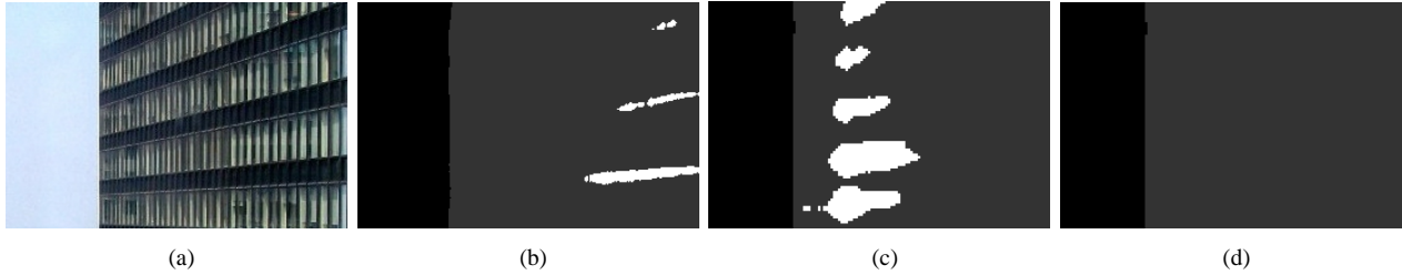
Fig. 3. Two-level texture map based on steerable filter decomposition. (a) Original grayscale image. (b) Texture classes at scale 0. (c) Texture classes at scale 1 (upsampled to original image size). (d) Combined texture classification.
