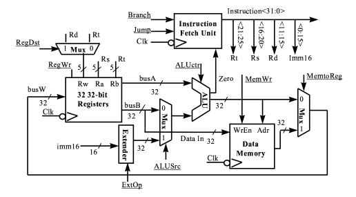
Use the schematic below to describe your changes. Show your connections and the values of the control signals (you may use add, subtract, etc. to describe ALUctr values rather than using binary numbers).
