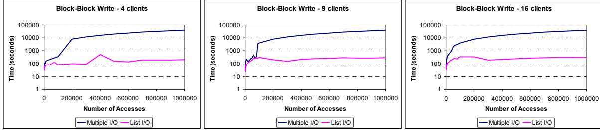
Figure 12. Block-block write results with various clients. These results are obtained by using 4-16 clients reading data with the block-block file access pattern.
