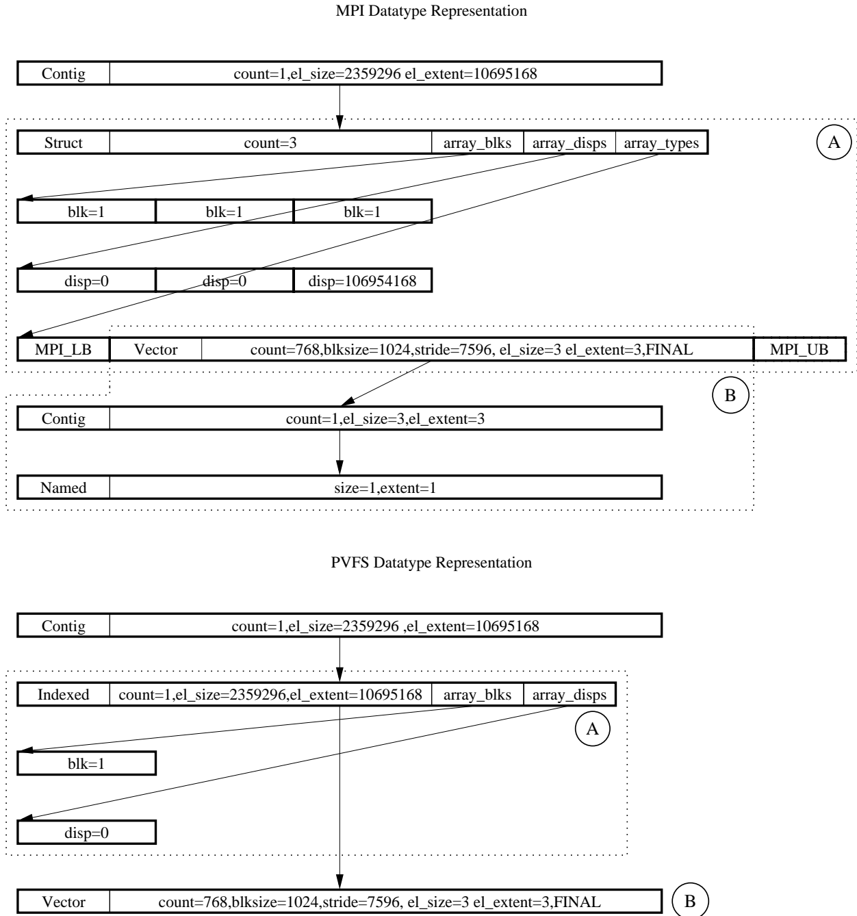
Fig. 7. Example tile reader file access pattern conversion. (A) shows how we convert a struct datatype into an indexed dataloop for performance optimization. This conversion eliminates the need for the MPLLB and MPLUB dataloops, making the dataloop representation smaller. (B) is an example of loop fusion in which we can merge datatypes into a single dataloop. The contig and named dataloops can be sufficiently described by the vector dataloop above them, eliminating the need for them.
