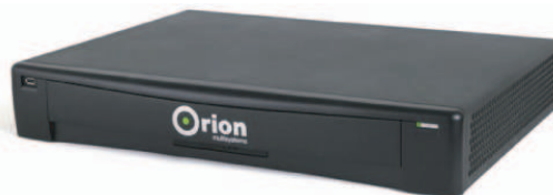
Figure 1. The DT-12 Personal Desktop Cluster Workstation.
