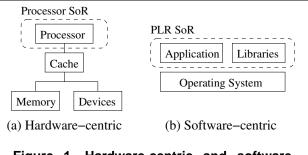
Figure 1. Hardware-centric and softwarecentric transient fault detection models.
