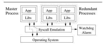
Figure 2. Overview of PLR with three redundant processes.
