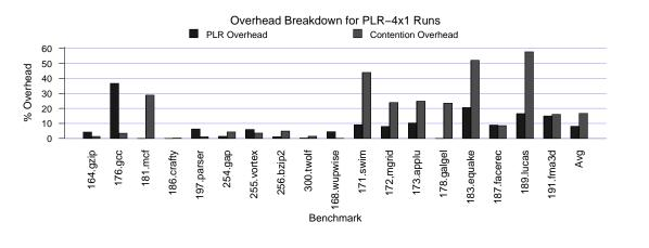
Figure 5. Overhead breakdown of running PLR on the a four processor SMP machine.
