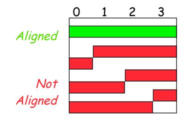
Alignment: require that objects fall on address that is multiple of their size.
