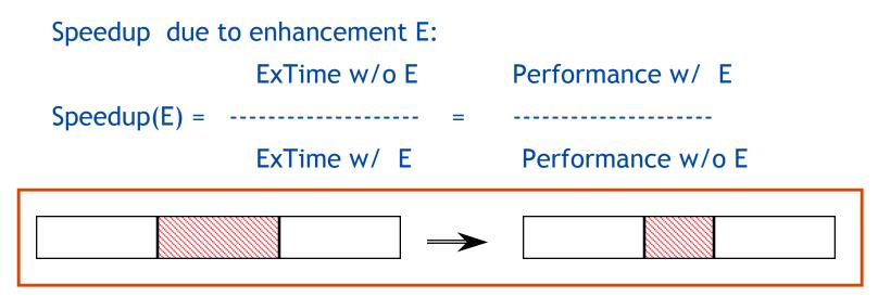
Suppose that enhancement E accelerates a fraction F of the task
