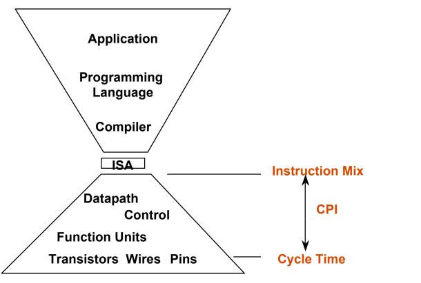
CPI is a useful design measure relating the Instruction Set Architecture with the Implementation of that architecture, and the program measured Principal Design Metrics: CPI and Cycle Time
