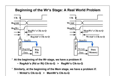
$^{\circ}$  We have a race condition between Address and Write Enable!
