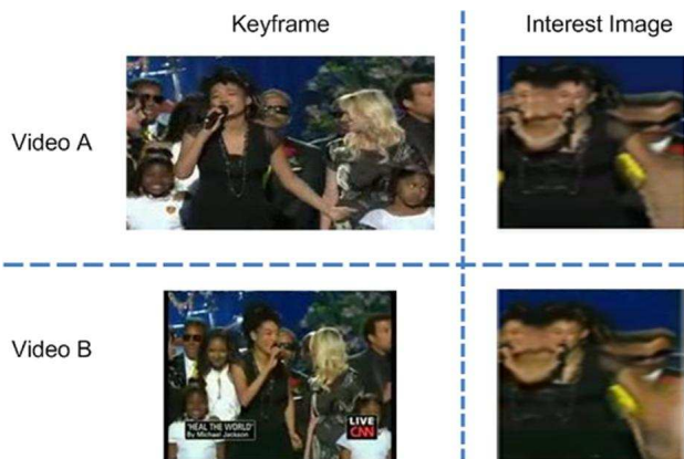
Figure 1. Key-frames and interest seam images from a pair of near duplicate videos. The key-frames contain same object with different poses which are difficult to match. In contrast, interest seam images are near duplicates which could be matched easily.
