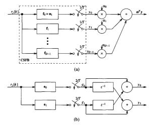
Fig. 2. (a) Detector with cyclically shifted filter bank.  $f_0, \cdots, f_{D-1}$  are cyclic shifts of the matched filter  $a_1$ . (b) Reduced complexity CSFB for D=2.
