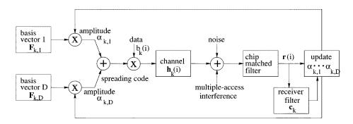
Fig. 1. Discrete-time baseband model for joint transmitter-receiver adaptation.
