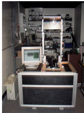
Figure 4.1: The picture shows the front of the display). A Fresnel lens is hoisted above the projection engine, and sits at about 5' above the ground.
