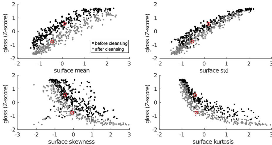
Fig. 11: Macro-scale perceived gloss versus surface statistics. The x-axis shows the normalized statistics of the surface reflection and the y-axis shows the normalized gloss scores after Thurstonian scaling. The circled points are the two original images of one subject.
