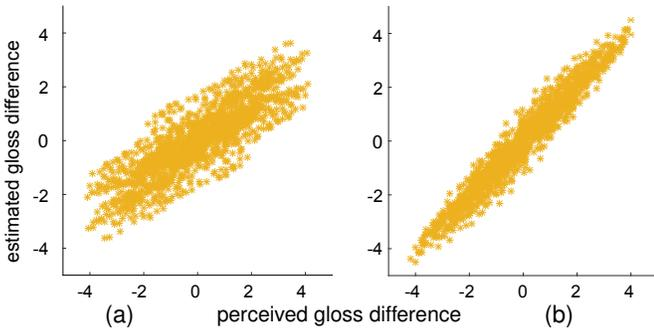
Fig. 13: Macro-scale Gloss: Prediction of relative gloss difference using statistical features extracted from (a) overall reflection (b) combination of separate surface and subsurface reflection images.
