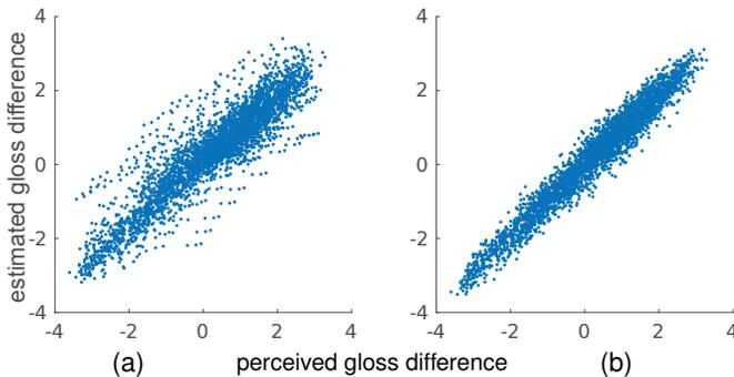
Fig. 16: Meso-scale Gloss: Prediction of relative gloss difference using statistical features extracted from (a) surface and subsurface reflection (b) subbands of surface and subsurface reflection images.
