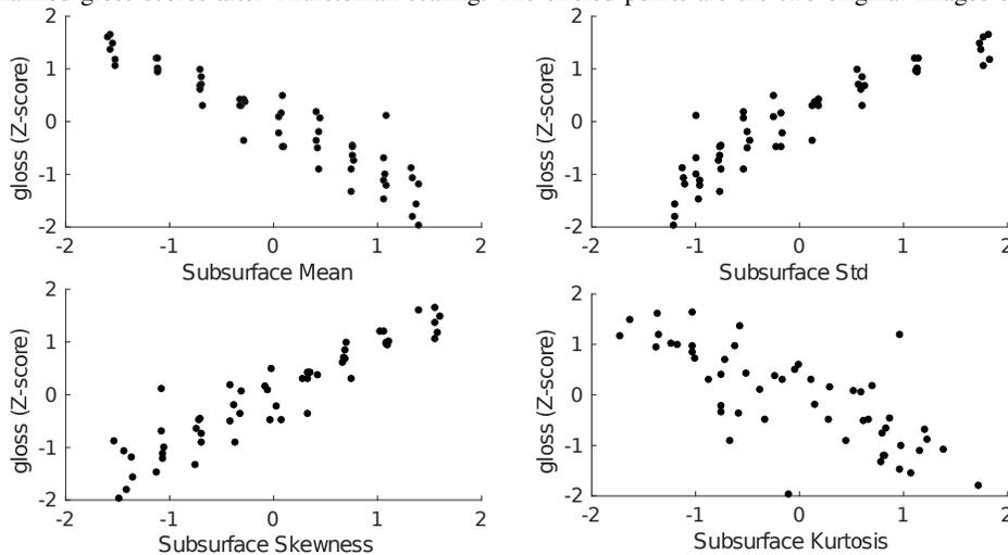
Fig. 12: Macro-scale perceived gloss versus subsurface statistics. The x-axis represents the normalized statistics of the subsurface lightness component and the y-axis represents the normalized gloss scores after Thurstonian scaling.
