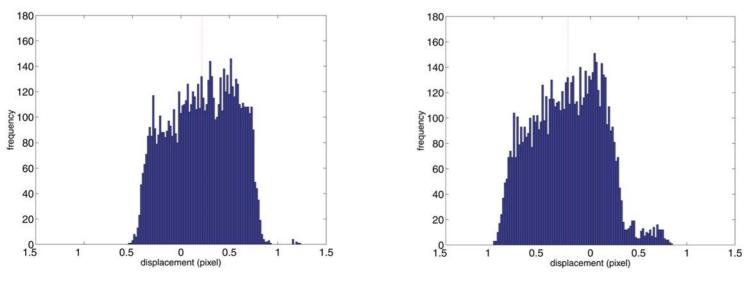
Horizontal displacement for even and odd rows of ink-jet printer
