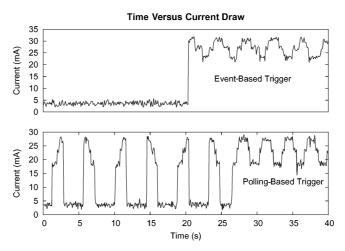
Fig. 4. External interrupt driven event-based query (top) versus polling driven event-based query (bottom).
