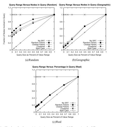
Fig. 9. Number of nodes participating in range queries of different sizes for different parent selection policies in a semantic routing tree ( $20 \times 20$  grid, 400 nodes, each point average of 500 queries of the appropriate size). The three graphs represent three different sensor-value distributions; see the text for a description of each of these distribution types.
