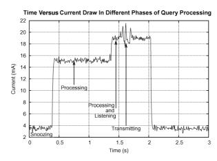
Fig. 3. Phases of power consumption in TinyDB.
