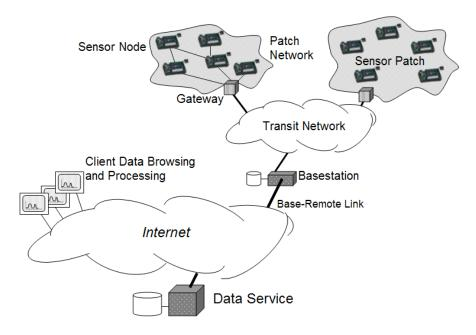
Fig. 12. System architecture for habitat monitoring.
