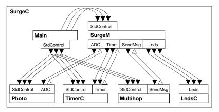
Fig. 5. The top-level configuration for the Surge application.
