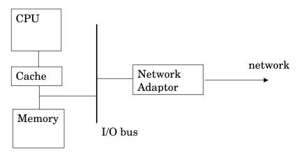
The physical layer and data link layer will generally be implemented in hardware on the Network Adaptor card this card is generally connected to the system I/O bus. Data is transferred to and from the host's main memory over the I/O bus.
