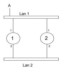
Suppose **node** A sends a packet with a destination address that is not in either bridges forwarding table. In this case, both bridges would forward to LAN 2. Each packet arrives at other bridge on LAN 2 and is forwarded to LAN 1, etc.
