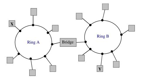
For X -> Y packet, bridge must receive packet from ring A and acknowledge packet, acquire token on ring B, and forward packet to Y.
