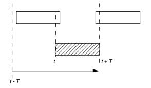
Thus the probability a frame is successfully transmitted,  $P_0$ , is the probability no other frames begin transmission during the contention window. This is the probability of 0 arrivals from a Poisson process with rate S, during 2 frame times. From the properties of the Poisson process (cf. Lec. 12), the number of arrivals in 2 frame times is a Poisson random variable with mean 2S. Thus
