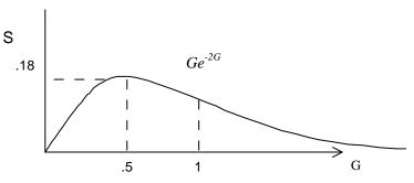
The maximum of this curve represents the maximum throughput for a stable system. To find the maximum we set the derivative of S(G) equal to zero as follows:
