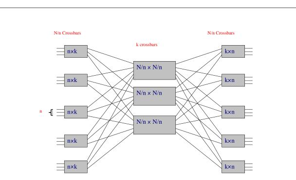
Suppose there are N incoming and outgoing ports. These are divided into N/n groups of n ports. Each group of n incoming ports is attached to a nxk first stage crossbar switch. The k output ports of each of these switches are connected to one of k second stage  $N/n \ge N/n$  switches. Finally there is a last stage of  $N/n \ge N/n \ge N/n \le N/n$  switches. An incoming call is switched through all 3 stages.
