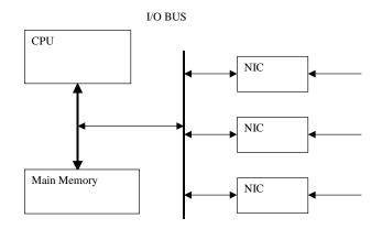
In this switch, when a packet arives, it gets transferred into memory. The CPU executes a routing table lookup for output port. The packet then gets transfered to the output NIC and forwarded. In this buffering is needed in the interfaces for each input, in case the I/O bus is busy. This design can be limited by the I/O bus speed, the memory bandwidth, or the CPU speed.
