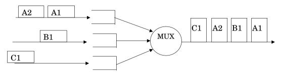
Statistical multiplexing is usually implemented at the packet level. Packets may have variable sizes or may all be a fixed size depending on the network. For example the Internet allows for variable packet sizes, while in ATM networks all packets have a fixed size of 53 bytes. The outgoing link may be synchronous and require each packet to be in a fixed slot, or it may be asynchronous allowing a packet to be sent at any time.
