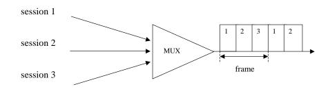
TDM is used with digital data. TDM was introduced into the public telephone network in the 1960's and has largely replaced FDM systems in the U.S.
