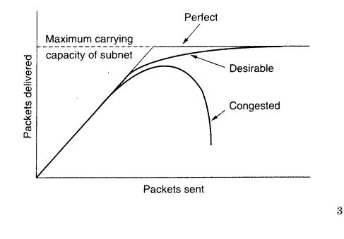
For example, originally the Internet (TCP/IP) did not implement congestion control. This led to a series of congestion collapses starting in 1986. In Oct. of 1986, the data throughput between Lawrence Berkeley Laboratory and UC Berkeley dropped from 32 kbps to 40 bps<sup>2</sup> [V. Jacobson, "Congestion Avoidance and Control", *Proc. of SIGCOMM '88.*] To avoid this type of behavior, congestion control was incorporated into TCP.
