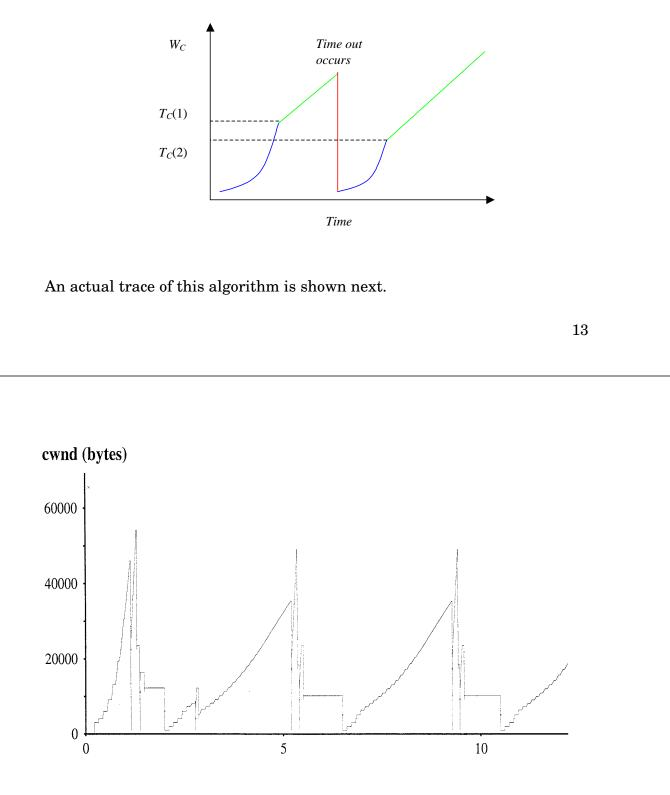
Again the vertical axis is the congestion window and the horizontal axis is time.
