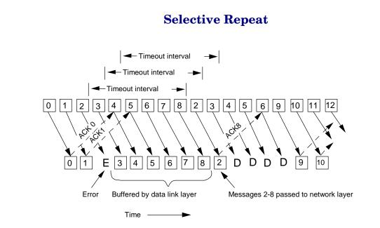
Notice that not all the frames sent in a timeout interval need to be retransmitted. (e.g. frames 7 and 8).
