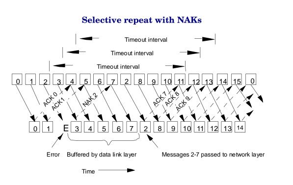
Notice that with NAK's it may be advantageous to set the timeout interval much longer than the round-trip time to avoid unneeded retransmissions.
