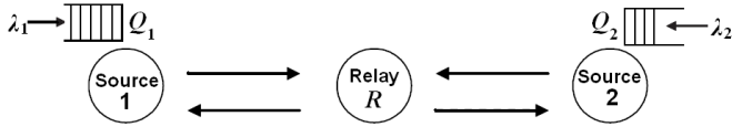
Fig. 1. Two-way relay network: Two sources with packet arrivals and a single relay to exchange the incoming packets.
