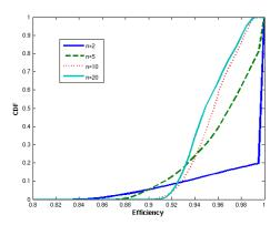
Fig. 5. Empirical CDFs of the efficiency of the two-user sequential allocation for the bandwidth auction with different n. The transmitted power  $P = 10^{-6}$  and  $d_0 = 50$  m.
