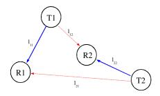
Fig. 3. Simulation scenario in which the location of the transmitter T1 is uniformly distributed within a circle centered at R2, and R1 and T2 are placed at random locations within circles centered at T1 and R2, respectively.  $(l_{11} \le d_0, l_{22} \le d_0 \text{ and } l_{12} \le d_0)$
