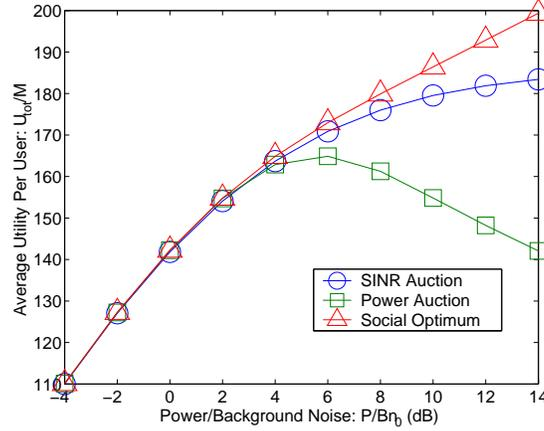
Fig. 2. Utility comparisons in a finite system of users with logarithmic utilities and co-located receivers:  $(Bn_0, M) = (10^2, 4)$
