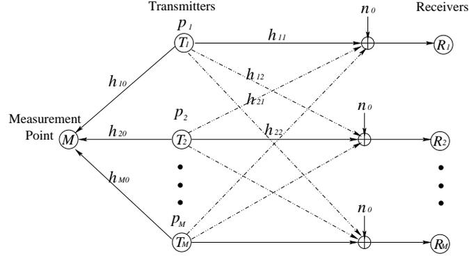
Fig. 1. System model for  $M$  transmitter-receiver pairs
