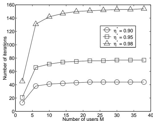
Fig. 5. Performance of the myopic bid updating algorithm with logarithmic utilities and co-located receivers: number of iterations required for a system with  $(P/n_0, B) = (10^4 M, 10^2 M)$  and different target  $\eta^*$
