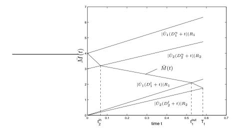
Fig. 2. An example of the time evolution of  $\bar{M}(t)$ ,  $|\dot{U}_i(D_i^u+t)|R_i$ , and  $|\dot{U}_i(D_i^l+t)|R_i$  for a two-class system. The intersections of  $\bar{M}(t)$  with the other curves correspond to the times  $t=0,t_2^{in},t_1^{out},T_f$ .
