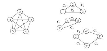
Fig. 6. Example graphs. On the left is the original graph G; on the right is the derived graph G' which has a maximum degree of 2. The two "children" of each node i in G are labeled by i and i' in G'. An edge coloring of G' using three colors  $(C_1, C_2, C_3)$  is also shown.
