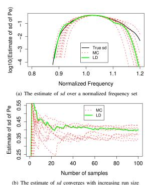
Fig. 5. The estimate of  $P_e$ 's standard deviation and its convergence for Icache: Comparing 1 LD to 10 MC runs with (a) Fixed run size of 100 samples. (b) Fixed clock frequency at 1.0.
