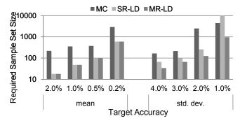
Fig. 6. The number of samples needed for targeting accuracy when estimating chip leakage power: MC, SR-LD and MR-LD.
