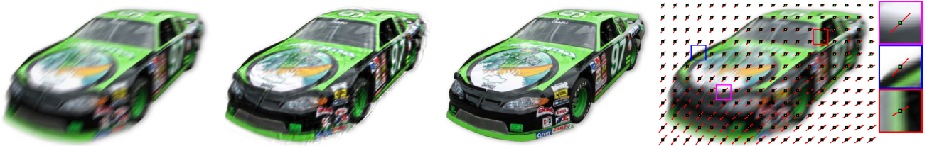
Figure 6. Affine motion from blur with synthesized data. Left to right: affine blurred image, deblur result, ground truth, visualized affine motion field estimation result with close-up views (please notice that the estimated local blur vector matches the blur extend precisely).
