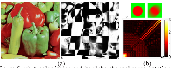
Figure 5. (a) A color image and its alpha channel representation \alpha , (b) top: original unblurred image ( 70 \times 70 ) and one blurred image with \mathbf{b} = (20, 20)^T , bottom: error ( \|\mathbf{b}^* - \mathbf{b}\| ) map of parameter estimation for all \mathbf{b} \in \{(u, v)^T \mid u, v \in \{0, 1, \dots, 30\}\} .
