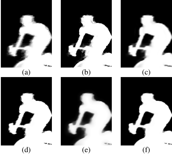
Figure 5. Comparison of \alpha estimation algorithms given \alpha_p and p (the estimated motion vector is (14, -3)' ), (a) noisy \alpha_p extracted by the matting algorithm, (b) result by the back-projection method [13], (c) result by deconvolution with sparsity prior [17], (d) our result without the edge smoothness prior term, (e) our result without the binary prior term, (f) result by our method (Eqn. 13).
