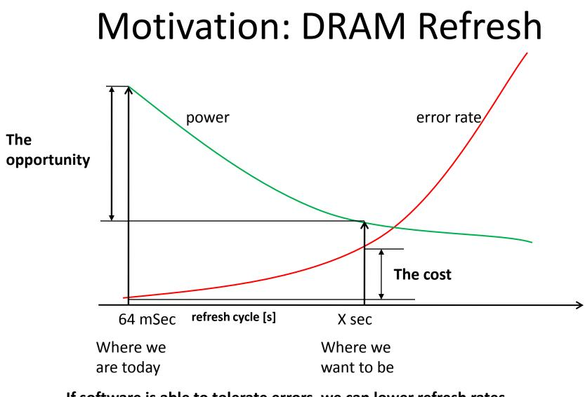
If software is able to tolerate errors, we can lower refresh rates pretty drastically to save power
