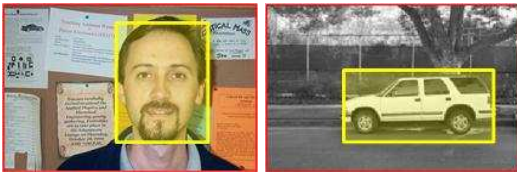
Figure 4: Evaluation of meaningful itemsets mining. The highlight bounding box (yellow) represents the foreground region where the interesting object is located. In the idea case, all the MI \mathcal{P}_i \in \Psi should locate inside the bounding boxes while all the meaningless items W_i \in \Omega^- are located outside the bounding boxes.
