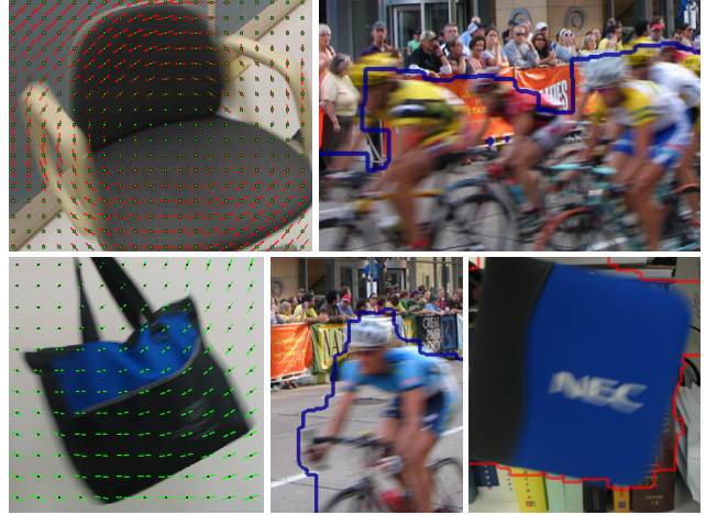
Figure 12. More results for space-variant motion from blur. The motion blur models for the top row: non-parametric, space-invariant plus non-blurred, bottom row: affine, space-invariant plus non-blurred, and rotational plus non-blurred.
