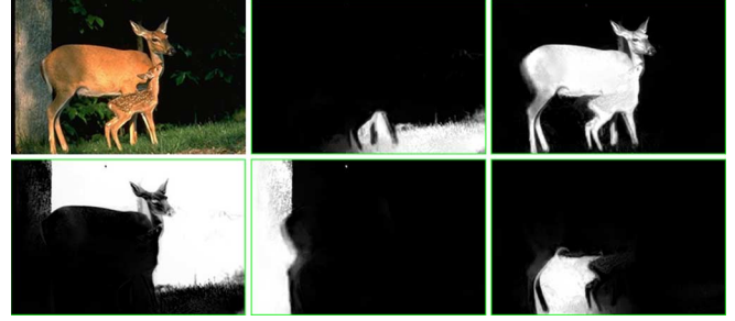
Fig. 4. Multiple layer image representation. The top left image is the input, the other five images represent the \alpha value for the five layers.
