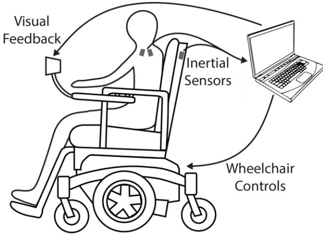
Figure 1. Diagram of the Body Machine Interface. Shoulder kinematics are recorded by inertial sensors, processed by an on board computer and commands are sent to the power wheelchair.
