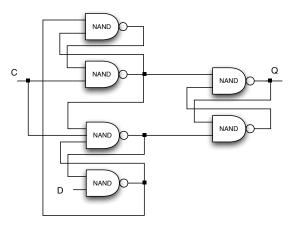
3. (20 pts) Is the following sequential circuit a Mealy machine or Moore machine? Why? Please give its state graph. Assume each gate or Flip-Flop has 10ps delay and the setup time for each FF is 5ps, what is the minimal clock period for the circuit to work correctly?
